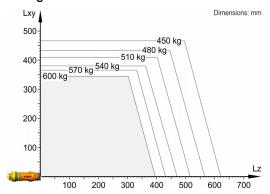
The KR 600 R2830 is designed for a rated payload of 600 kg in order to optimize the dynamic performance of the robot. With reduced load center distances, higher loads up to the maximum payload may be used. The specific load case must be verified using KUKA.Load. For further consultation, please contact KUKA Support.
