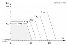
The KR 10 R1420 is designed for a rated payload of 10 kg in order to optimize the dynamic performance of the robot. With reduced load center distances, higher loads up to the maximum payload may be used. The specific load case must be verified using KUKA.Load. For further consultation, please contact KUKA Support.
